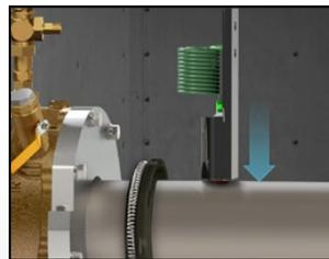
The Duramax® DryMax® Shaft Seal System includes an earthing assembly to help prevent shaft corrosion. The assembly contains a replaceable carbon brush that is spring loaded and grounded to the ship's hull.
