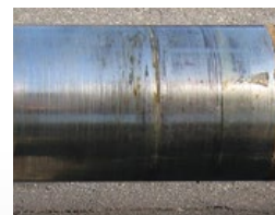
Shaft scoring caused by flax packing
